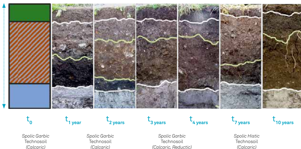
FIGURE 19. How the horizons of a technosoil evolve over time. ©Schwartz, G. Séré, Université de Lorraine
